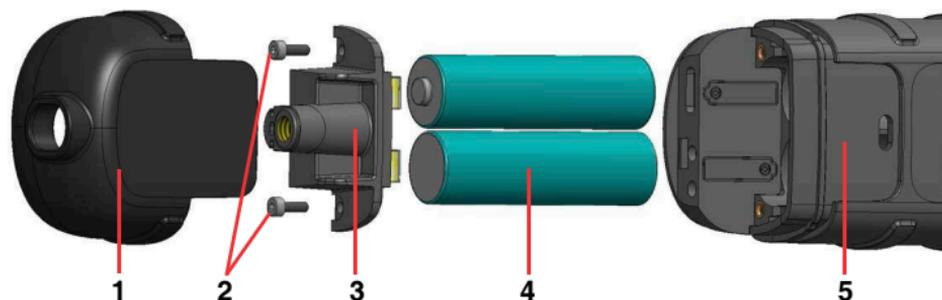
Figure 4: RadMan 2 battery compartment
