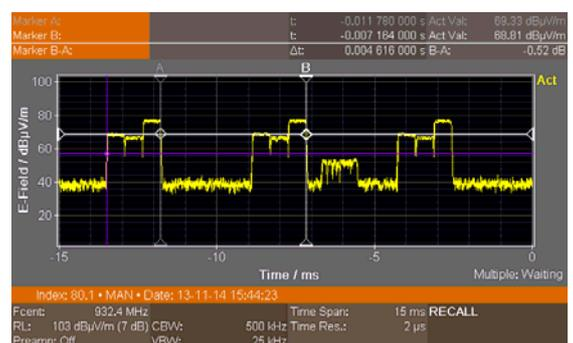
**A GSM downlink signal shown in Magnitude display mode, triggered on the rising edge. Time resolution is 2 µs. The 546 µs timeslots can be clearly seen and the frame duration can be measured using markers A and B: Δt = 4.616 ms.**
