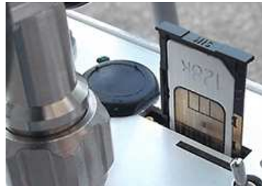
Fig. 4-10 SIM card installation
