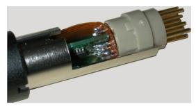
Figure 3: A small memory chip in the NBM probe stores all the major probe data
