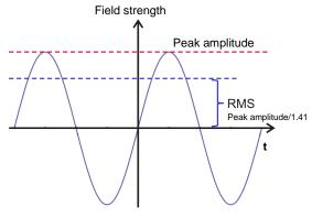
Figure 1: RMS value of a sine wave field strength signal versus time
