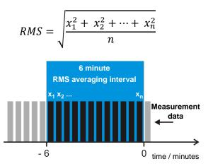
Figure 4: Formation of the floating average field strength value using a continuous result memory
