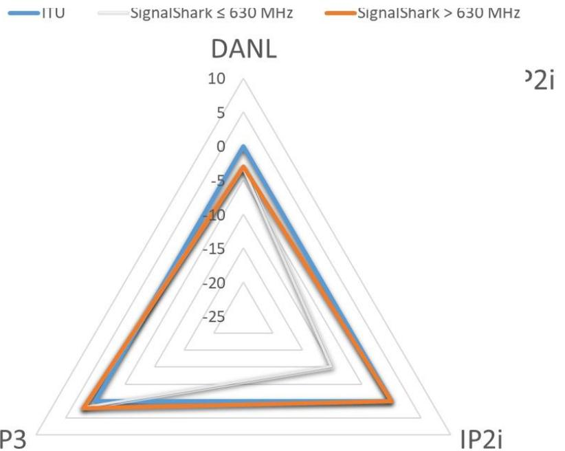
Figure 23: SignalShark dynamic range parameters compared with the ITU recommendations
