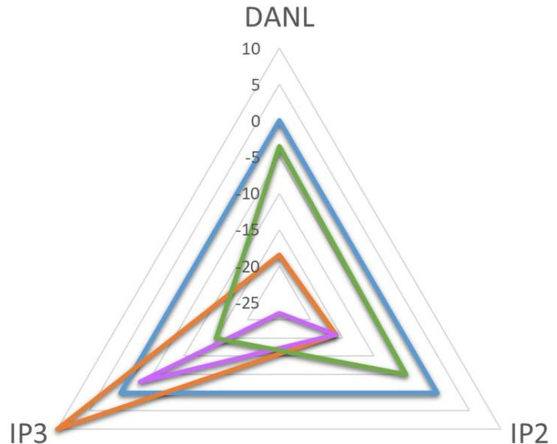
**Figure 4: Specifications of Anritsu MS2720T (orange), R&S FSH (violet), R&S PR100/DDF007 (green)**
