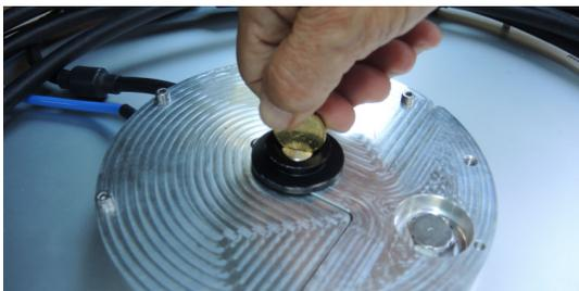
4. Mount the adapter with the ADFA to the tripod head:
