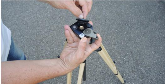
3. Attach the adapter to the ADFA at the center hole (see red marking on the picture below) and tighten it with a suitable tool (for example, screwdriver, coin).
