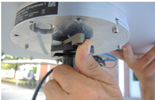
**CAUTION!** The ADFA is heavy. Be careful when mounting the ADFA on the tripod.
