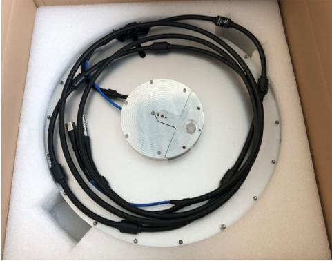
Figure 1: Package with an ADFA and RF cable already connected.
