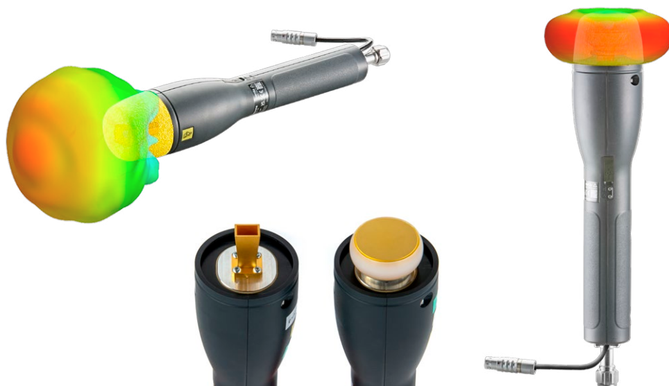
Figure 2.4: SRM-antennas for the millimeter wave range (left: Horn antenna for directional reception; right: dipole antenna for omnidirectional detection). The angle-dependent reception characteristic of the antennas is visualized by a color representation.
