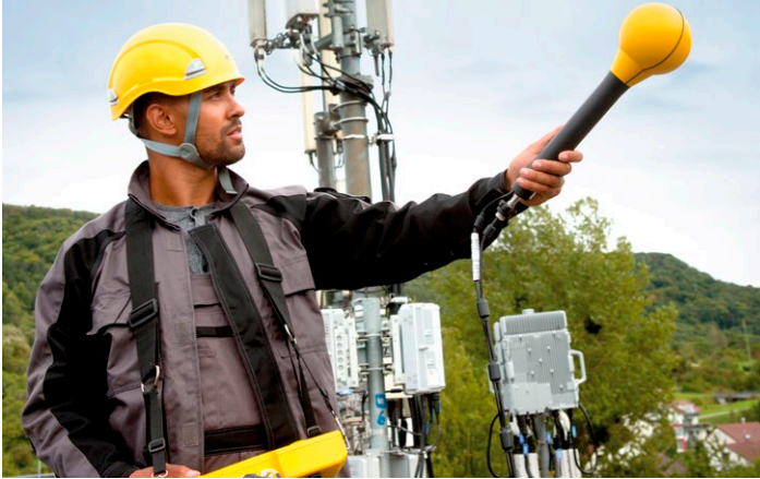
Figure 2.1: Using the SRM-3006 on an antenna roof.
