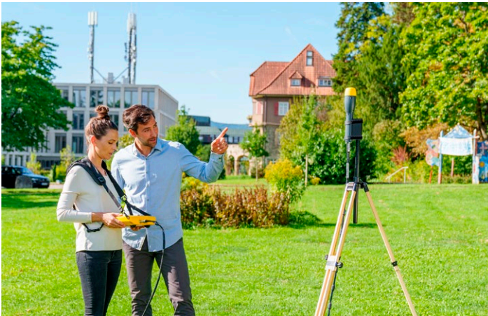
Figure 2.2: Field strength measurement using a separate antenna mounted on a tripod.
