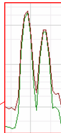
Figure 1: Result of a spectrum analysis in the VHF range. The small difference between the maximum and average values is typical for FM radio broadcasts.
