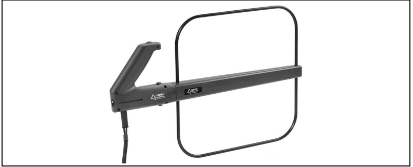
Figure 7: Loop antenna, frequency range 9 kHz to 30 MHz
