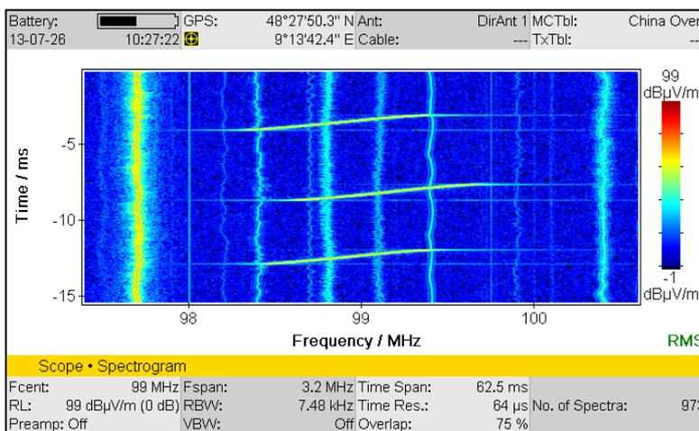
*A gapless spectrogram covering 15 ms. The interference appears roughly every 3.8 ms and takes about 0.8 ms to move from a lower to a higher frequency across a variable bandwidth.*
