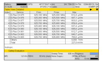
Figure 3: Safety Evaluation with resolution down to individual channel level. A prerequisite here, too, is that a corresponding Service Table has been recorded.
