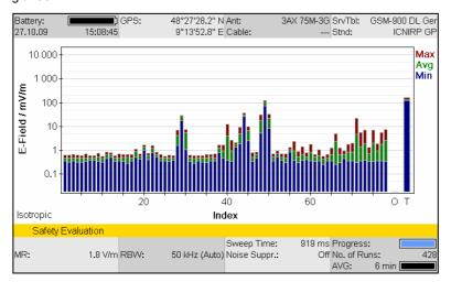
Figure 4: Safety Evaluation of individual channels shown as a bar graph. The bar to the right represents the overall value (Total).
