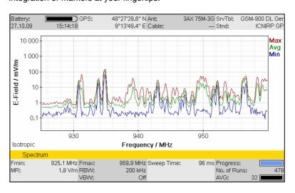
Figure 5: Spectrum analysis. When you switch from Safety Evaluation mode to Spectrum Analysis mode, the instrument automatically retains the frequency limit settings.
