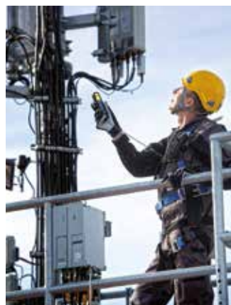
The RF Detection Mode (RadMan 2XT) can be used to quickly and simply check that an antenna has been switched off
