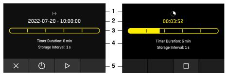
Fig. 9: Progress display via time bar: Activated timer (left), after start (right)
