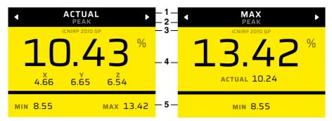
Fig. 13: Numerical display in the SHAPED TIME DOMAIN operating mode
