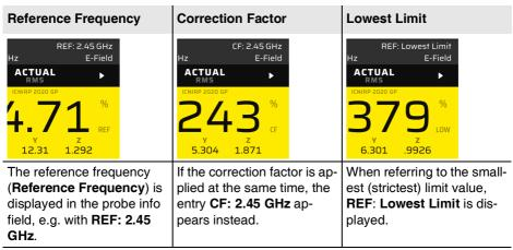
The standard selected in the menu is also shown in the display (in the yellow field above the isotropic measured value).
