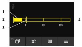
Fig. 4: Bar display in the FIELD STRENGTH operating mode
