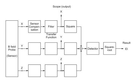
Figure 1: In weighted mode, the signal outputs are taken after the weighting filter
