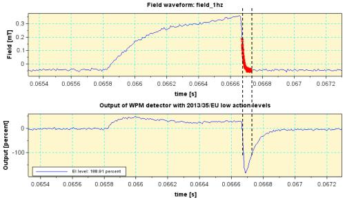
Figure 6: Time comparison of field waveform and weighted output for one pulse
