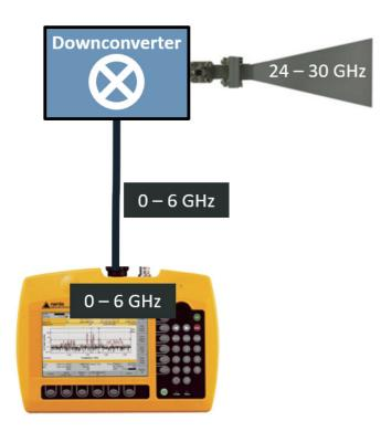
It's down converting mm-Waves into mid-frequency range so that the signal can be more easily transported and processed.
