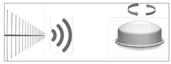
Fig. 5. The antenna is rotated in the test field at different frequencies to determine the catalog.
