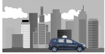
Fig. 6. The closer that the test vehicle gets to the source and the higher the source is in relation to it, the angle of incidence of the signal on the antenna is no longer horizontal but is at an angle from above, the elevation angle.
