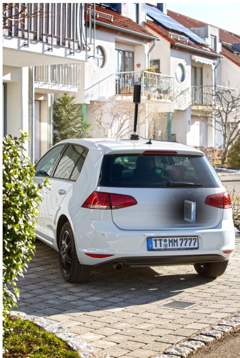
The fixed network installation can be expanded if required by means of mobile TDOA or AOA stations. This is illustrated here by fitting an omnidirectional antenna onto the roof of an automobile by means of a magnetic base. The SignalShark Remote Unit is fitted in the trunk. This setup is also excellent for independent spectrum monitoring or coverage measurements.
