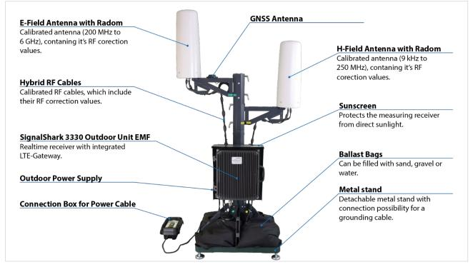
Fig. 1. SignalShark EMF measuring station
