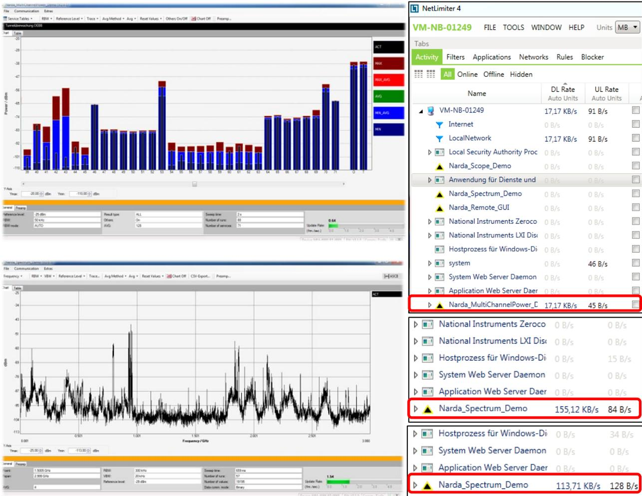
**Figure 4: Comparison of Data Rates in Multi Channel Power Mode (17 kByte/s) and Spectrum Mode Software (avg. 130 kByte/s)**
